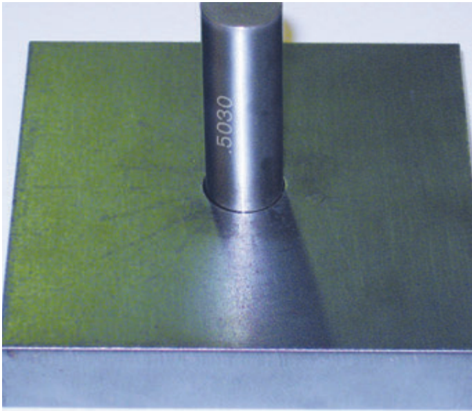
1 2 hole without True Hole technology cut with HPRXD Plasma
