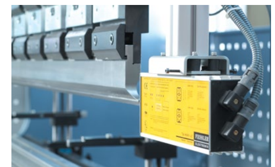
Ce Laser Safety System
